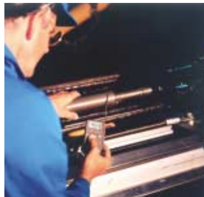
The ideal temperature on the coupling should be down to 60°C for air flushing and 45°C for water flushing.
