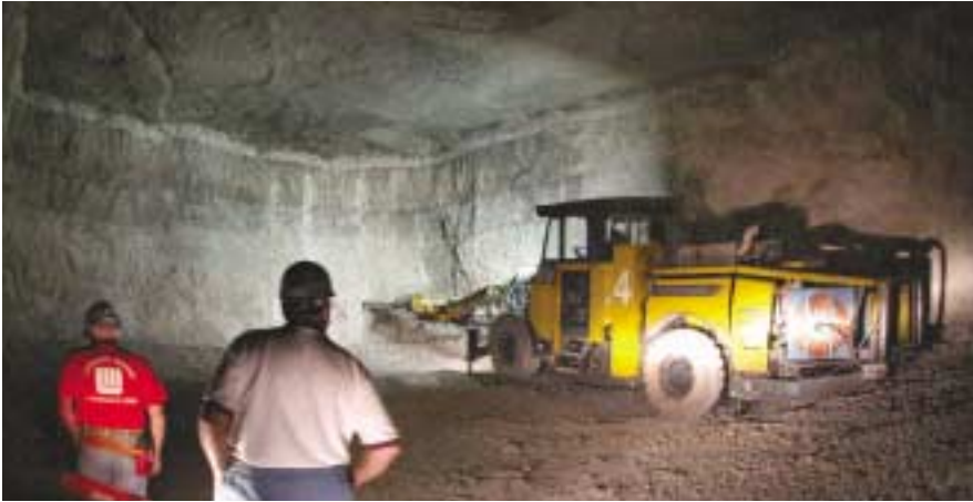
Rocket Boomer L1 C-DH drillrig at Linwood Stone.
